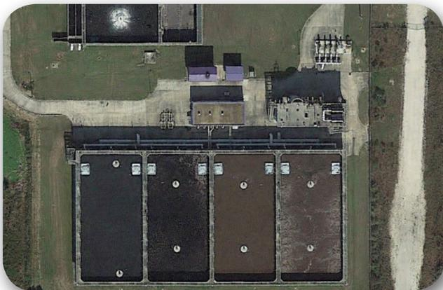
The AquaSBR® system at Sulphur started operation in March 2008. As population increased, it was found that the existing 30-year-old activated sludge plant was in need of a significant upgrade. The new system is a 4-basin SBR system fed by 29 pump stations located throughout the city and also receives septage from local haulers.
