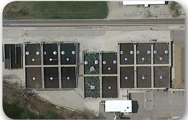
The Newburgh treatment plant was updated in 2000 to a 5-basin AquaSBR® system, designed to treat a maximum day flow of 9.4 MGD and a peak hour flow of 14.8 MGD. In 2010, three additional reactors were added to handle a maximum day flow of 14.9 MGD and a peak hour flow of 19 MGD.
