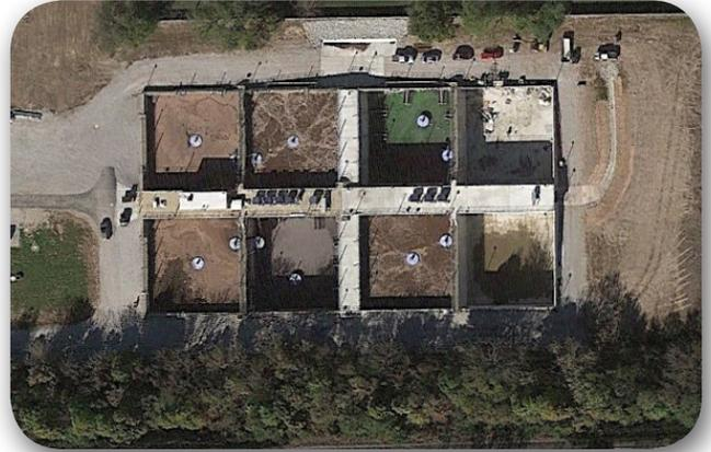
The West Central Conservancy District (WCCD) in Hendricks County, IN was established in 1992 and comprised of 5 geographical locations. An expansion in 2005 included the installation of a 4-basin AquaSBR® system which has the capacity to treat a much larger capacity (up to 8 basins) in a small footprint on the available land space.
