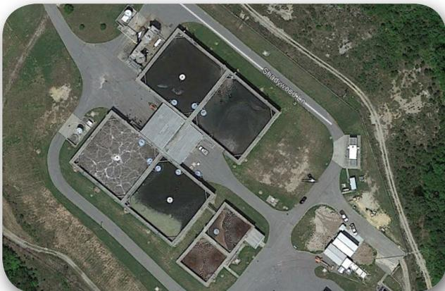
The Broad River WWTP consists of a 4-basin AquaSBR® system. One of the main drivers for the technology selection was the system's biological phosphorus removal capability. The plant started up in October 2008.
