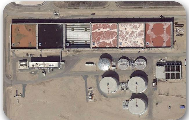
Operated by the City of Tulare, the Tulare Industrial WWTP is surrounded by rich farming communities. The 6-basin AquaSBR® system treats primarily industrial processing waste from six large milk processing facilities. This plant is one of the largest industrial SBR systems in the nation and provides quality recycled water to the Tulare community.
