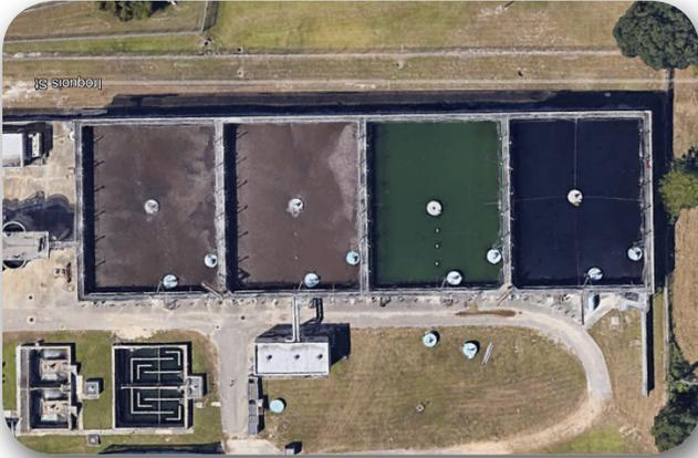
To accommodate increased growth, Keegans Bayou replaced an old trickling filter system with an AquaSBR® system. The expansion tripled the plant's capacity and services all of east Biloxi including an area of casino-hotel chains.
