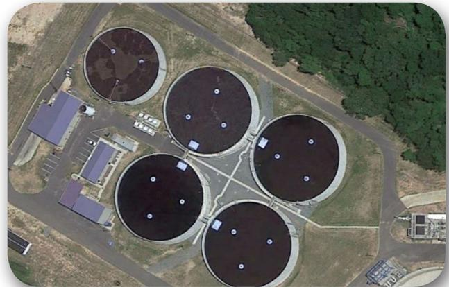
The Withlacoochee plant was designed after disastrous flooding was experienced by the old plant in April 2009. The new plant is situated outside of the flood plain at a 60 foot higher elevation than the old plant. The new SBR system assists in the successful handling of high flow rainstorm events by preventing the overloading of units downstream.
