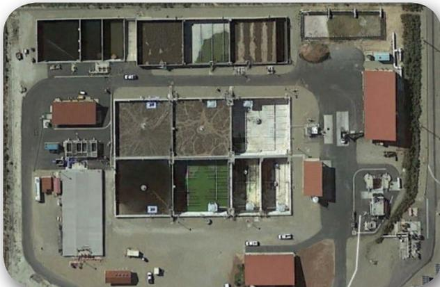
The Camp Pendleton AquaSBR® system was built in phases, starting in 2006 with 4-basins, then expanding in 2013 with the addition of two SBR reactors. One of the main drivers of the system was the turn-down capability with the ability to operate with seasonal flows and loadings.
