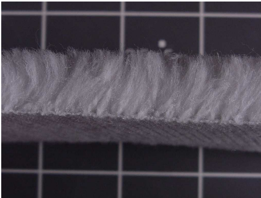
Figure 1: Magnified Cross Sectional View of Pile Cloth Media
