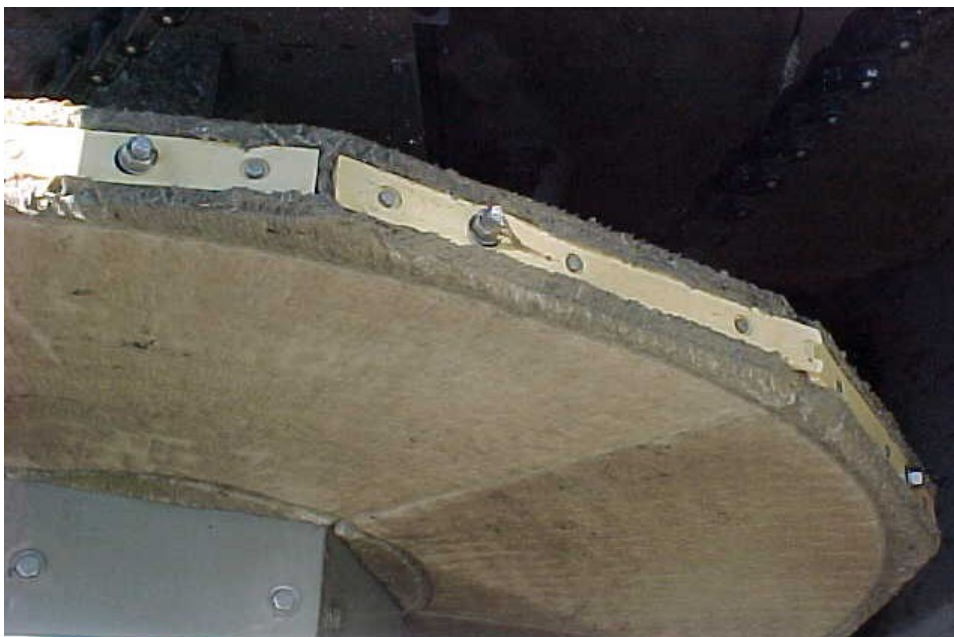
Figure 3: AquaDisk® Filter with Pile Cloth Media
