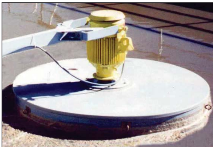
A typical 3 HP AquaDDM ® mixer
