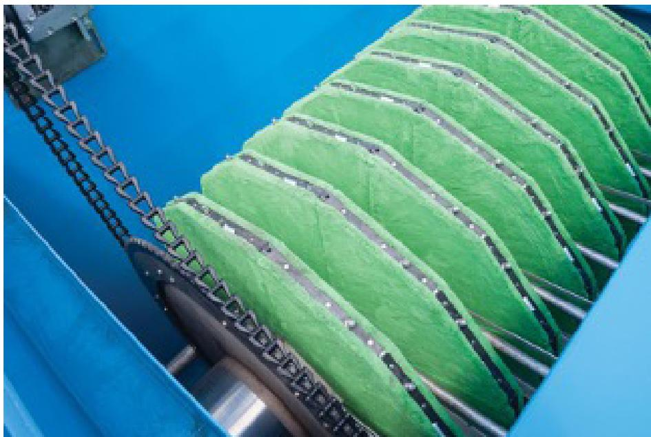
blinds, an automated backwash kicks on based on headloss. Backwash shoes make direct contact with the cloth media and remove solids using vacuum, which results in the water being filtered to be pulled back through the cloth for cleaning. The backwash waste can be pumped back to a waste-handling facility, such as thickener or the head of the plant in wet weather treatment applications.
