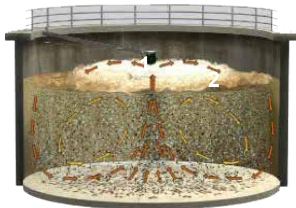
Typical Aqua-Jet® aerator operation.
