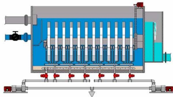
*Cloth media disk filters require about one-fourth the space because of the vertical orientation of the filter surface area.*
