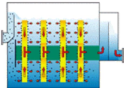
*Solids accumulate on the surface of the cloth disk and a backwash pump periodically pumps the solids out while the filter remains in operation.*
